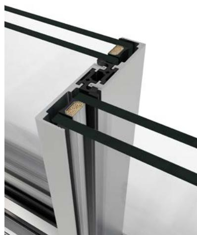
Sliding system with Thermal Break of avant-garde design seeking maximum brightness with the minimum amount of seen aluminium interlock in the market (only 20 mm) and allows enclosing large openings of up to 13.2 (width) x 3 (height) metres in 6 sashes.
